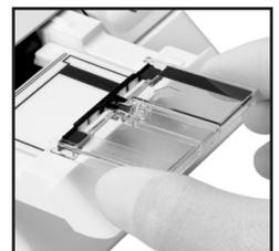
Note: From the time the cassette is open to the time the "RUN" button is pressed to begin the test, should ideally be less than 2 minutes.
